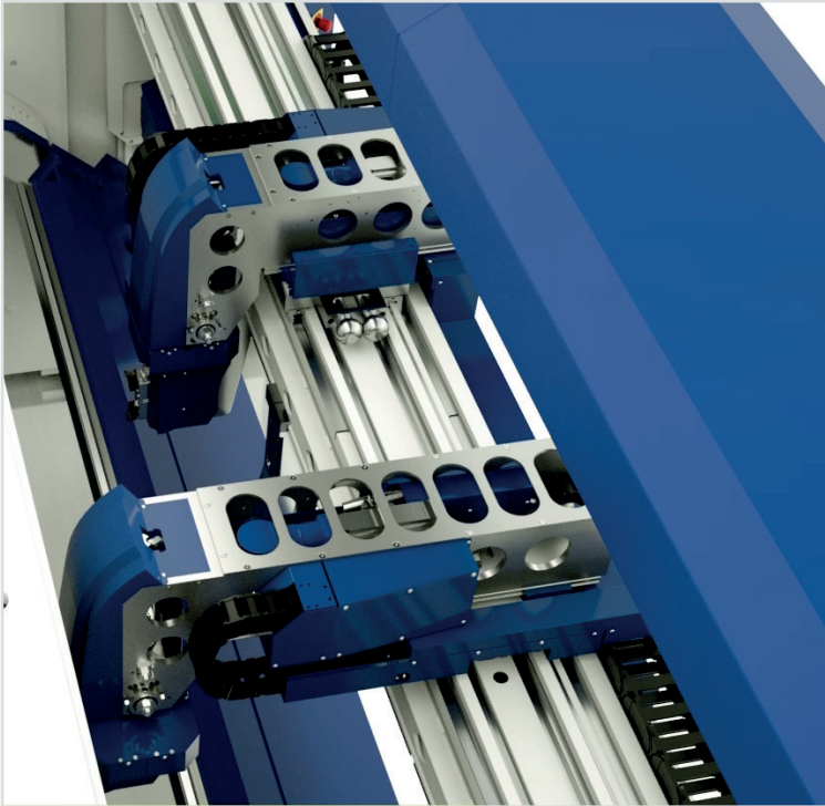
Two asynchronously movable tool changers each have a gripper unit.
