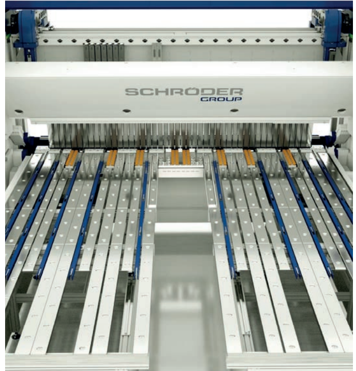
U-shaped back gauge with suction cups, controlled via POS 3000.
