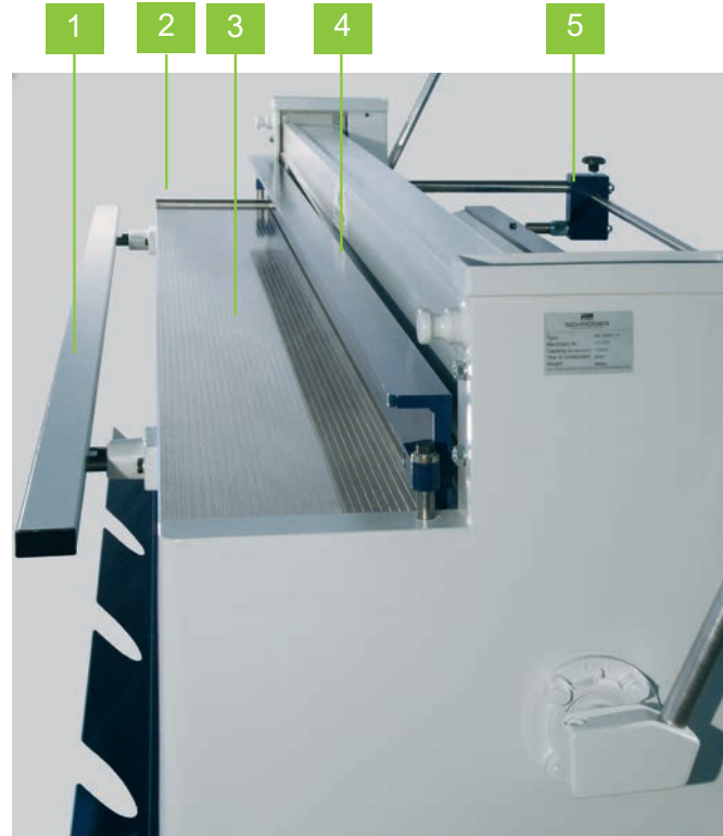
Manual back gauge with scale and handwheel adjustment [6] on the angle guides [5] for parallel and conical cuts.
