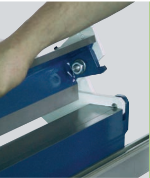
BAM 1000: Rotating clamping beam
