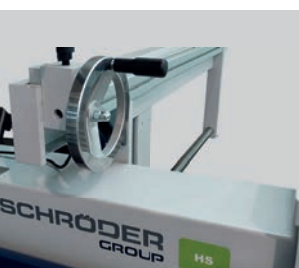
Optional: Manual back gauge 750 mm adjustable from the front with digital readout
