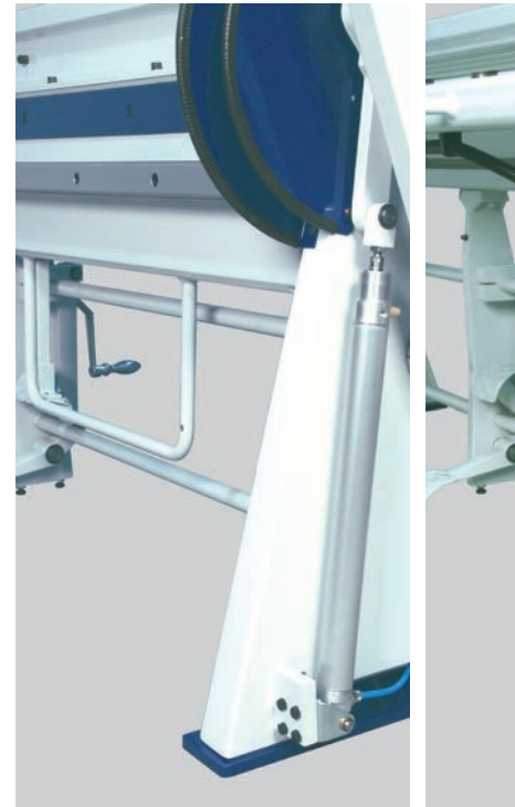
The pneumatic bending support is controlled by a finger lever on the folding beam handle.
